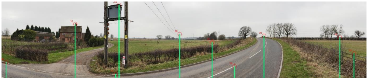
Figure 2: Camera matching CAD data within photograph
