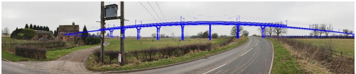
Figure 4: Model within image prior to blending and rendering
