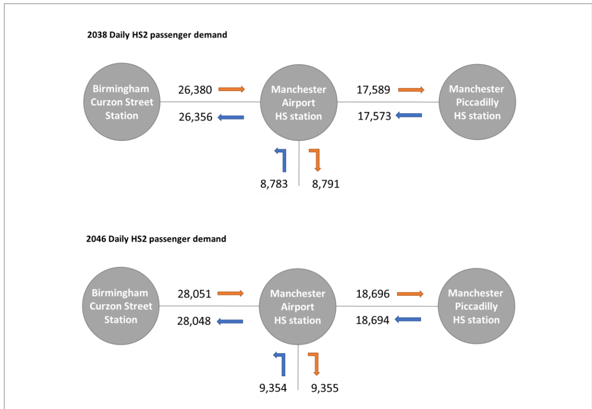
Figure 18-55: Daily HS2 demand at Manchester Piccadilly Station and Manchester Airport HS2 Station
