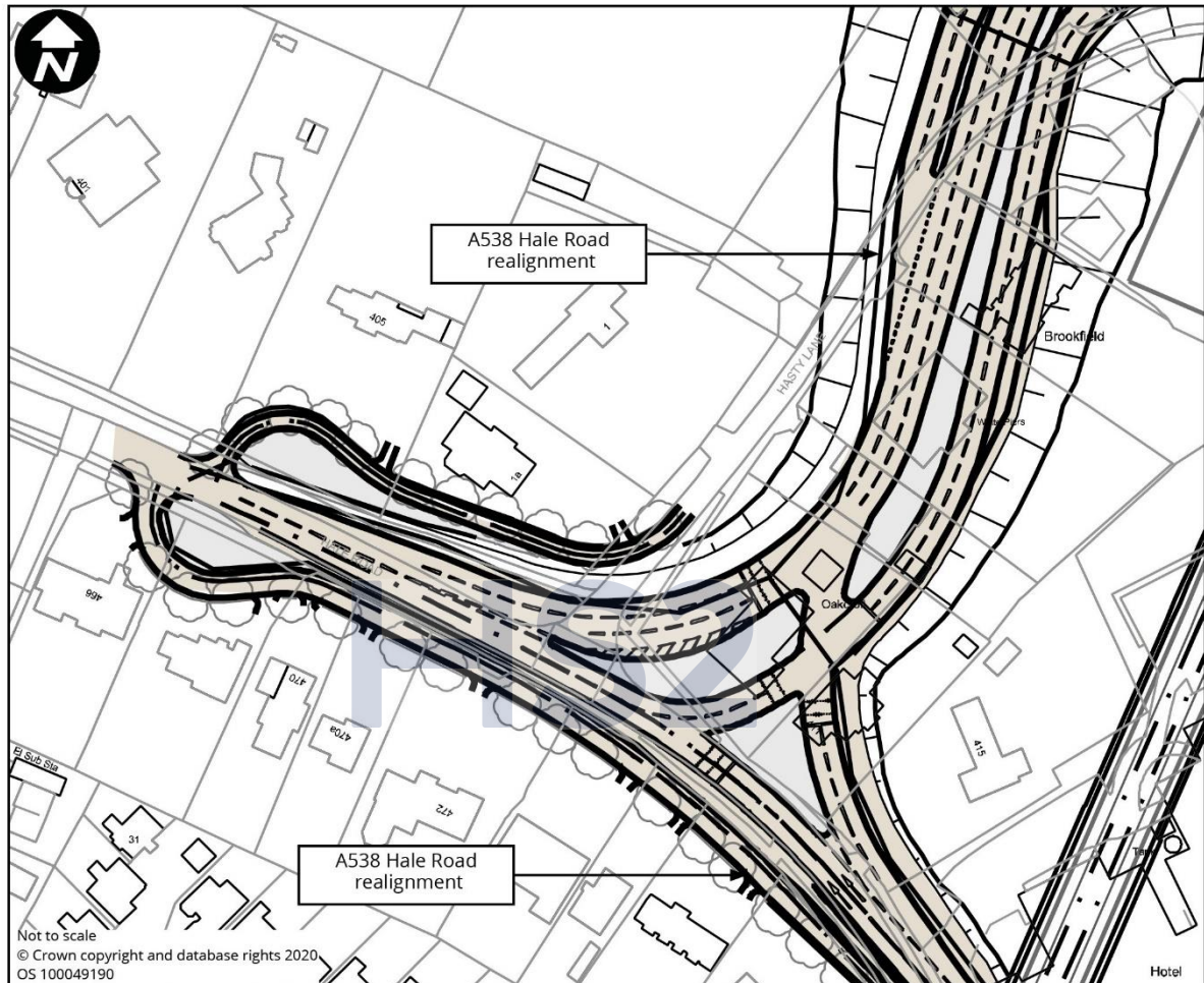
Figure 18-93: Junction layout diagram (A538 Hale Road/A538 Hale Road realignment)
