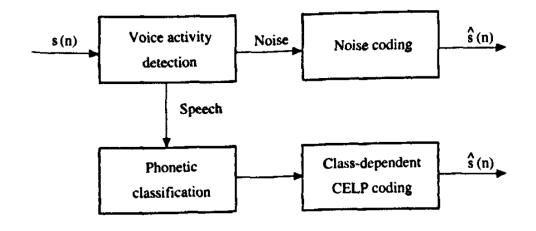
"Since VRPS is a CELP-type coder, the excitation parameters are shape vectors and gains selected from appropriate codebooks using an analysis-by-synthesis search technique. The properties of each shape codebook are determined by the properties of the phonetic class to be coded."
