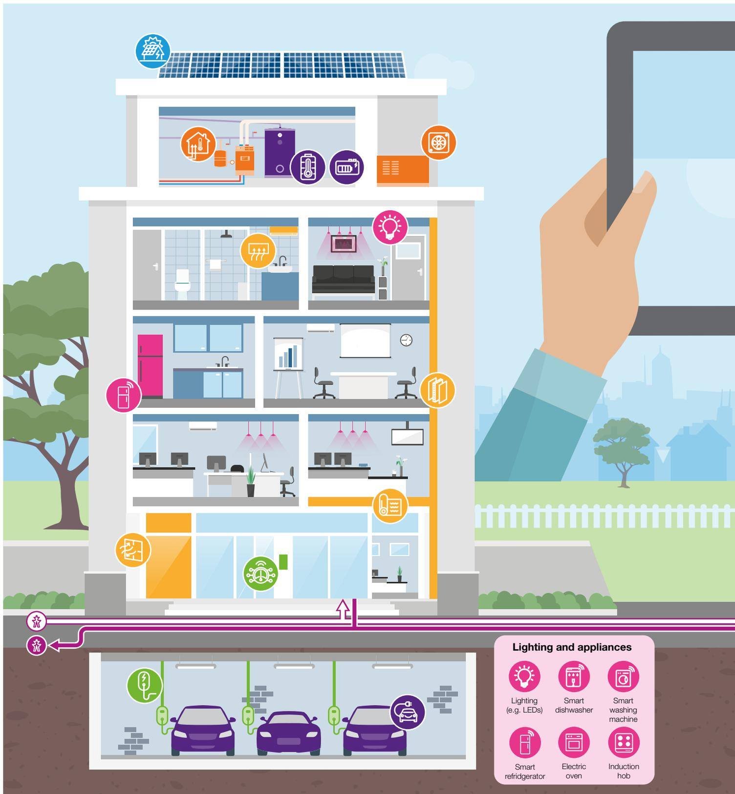
Figure 6 demonstrates an example of how buildings in the future may be designed to use and store energy in a more efficient integrated way. Key elements include: the use of a low-carbon source of heat, measures to ensure high thermal and energy efficiency, and the use of smart technologies.
