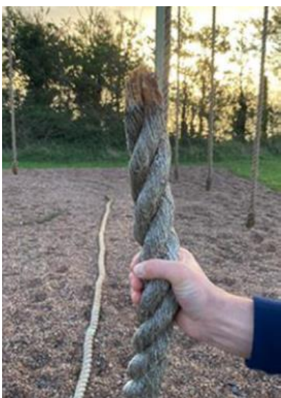
Failed natural hemp climbing rope
