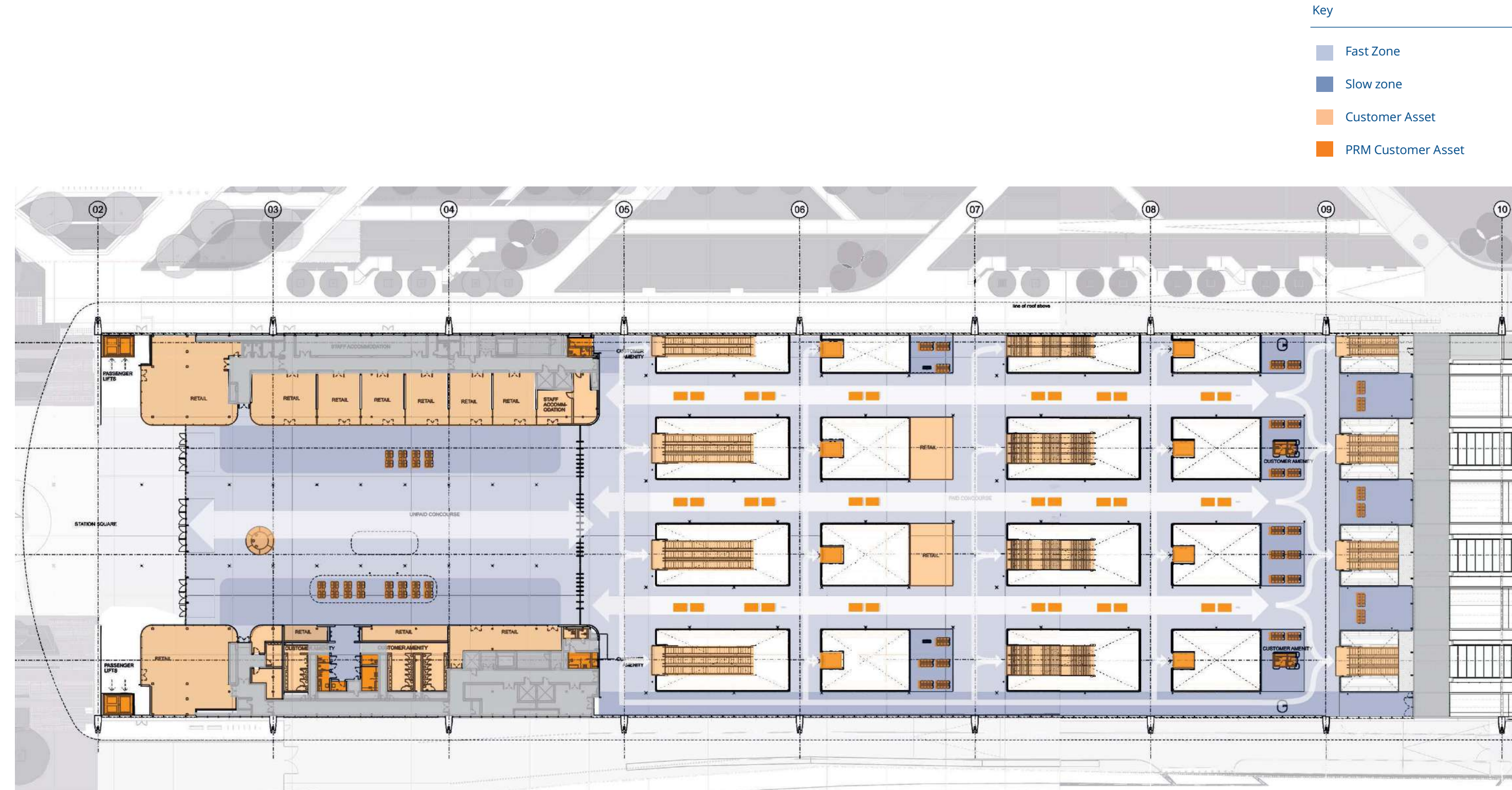
Fig.6.2 Diagram to show main flows of pedestrian customer traffic throughout the western concourse
