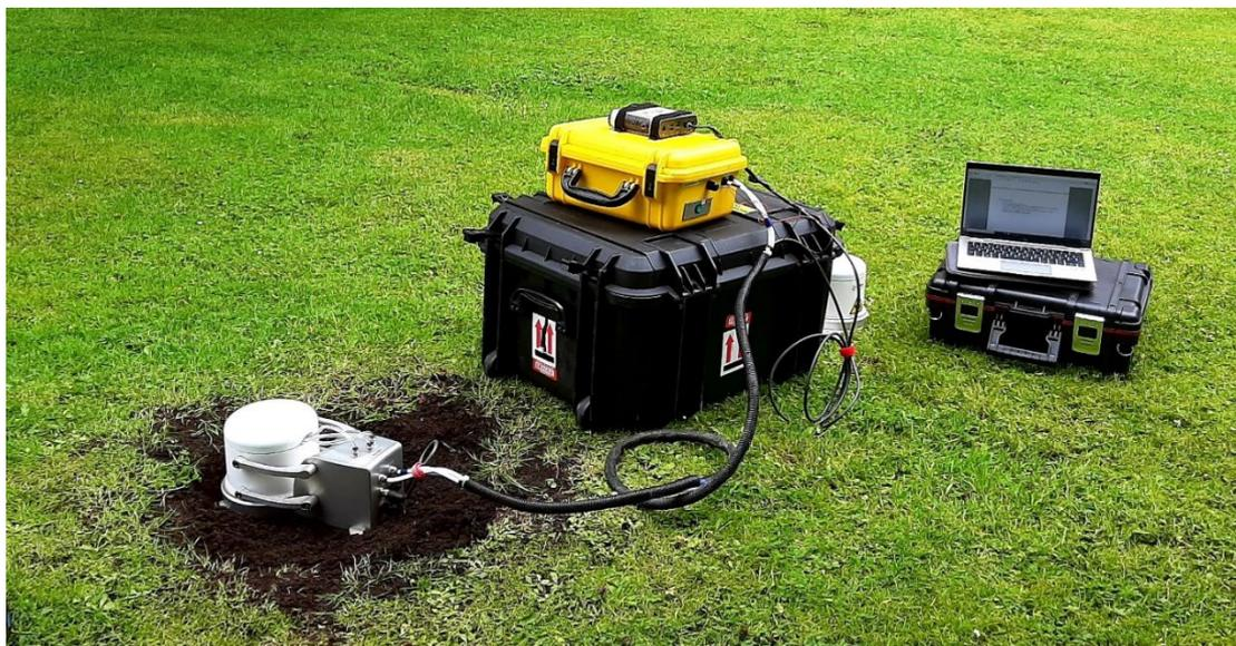
**Figure 3:** Testing of CH<sub>4</sub> dynamic flux chamber system prior to field campaign 2.
