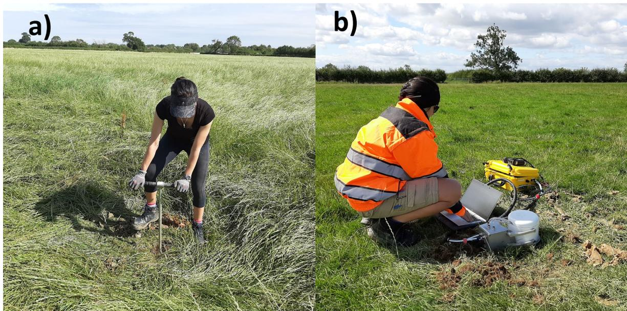
**Figure 4 a)** Shallow auger drilling at Long Clawson-1. **b)** CH<sub>4</sub> flux measurements being attained over a shallow auger hole (>2m deep) at the assumed decommissioned wellhead at Old Hills-1.
