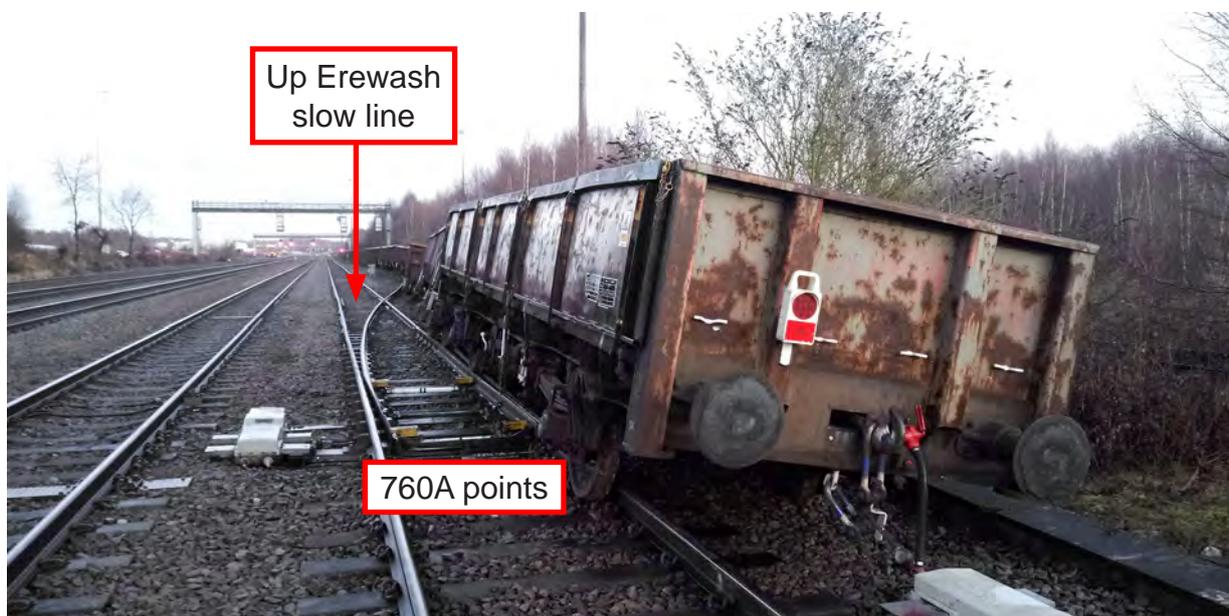
Figure 4: The derailed wagons (courtesy of DB Cargo)
