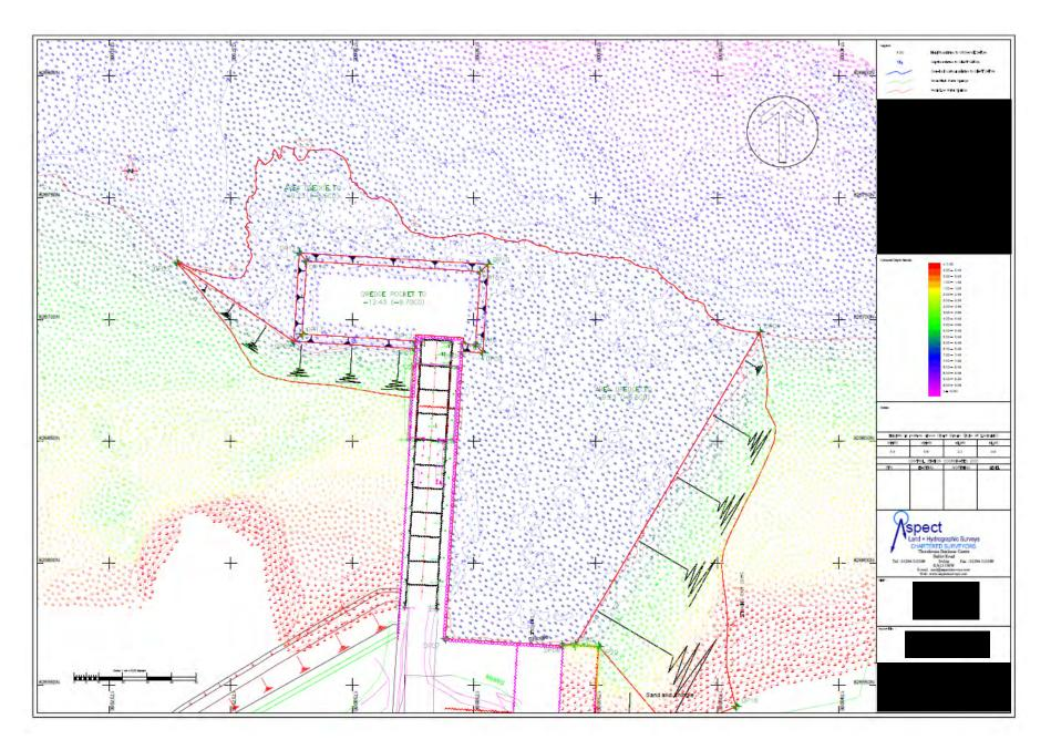
Enclosure 1 - Post dredge MBES survey Kyleakin pier Isle of Skye
