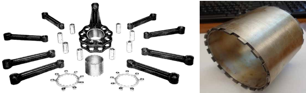
Figure 10 Master connecting rod assembly (Pratt & Whitney) Master rod bearing (Photograph used with permission)
