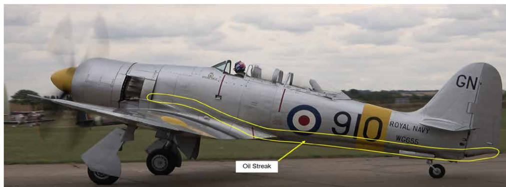
Figure 6 G-INVN after the first flight showing an oil streak on the left side (Still photograph taken from video used with permission - Sky High Films)
