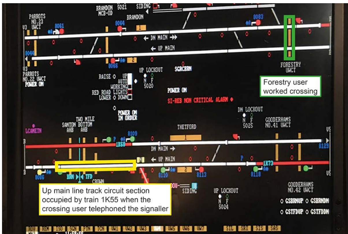
The Thetford workstation screen. Note that this image does not represent the situation at the time of the incident (image courtesy of Network Rail)
