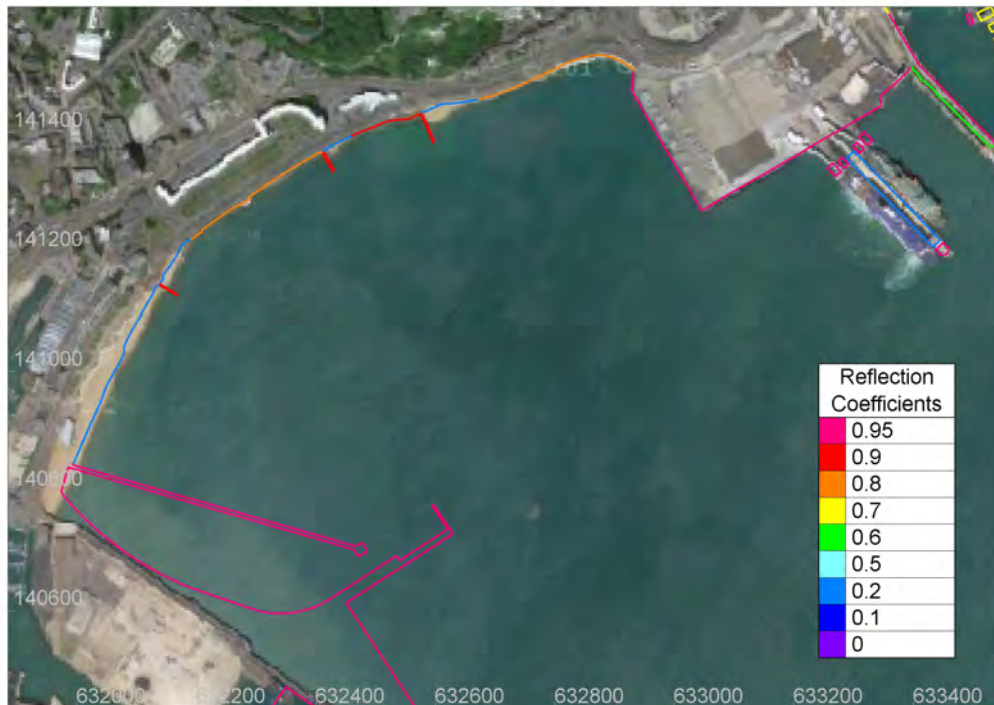
Figure 3.10: Reflection Coefficients (Sections A+B+C partially renourished)
