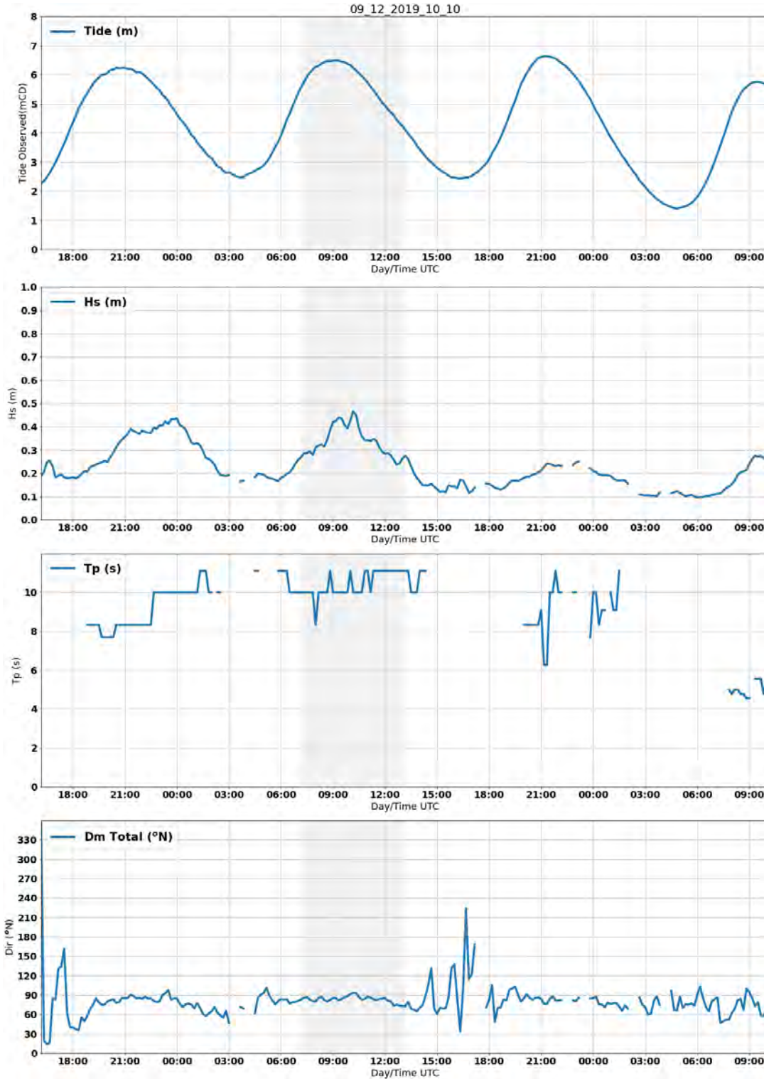
Figure B.6: Water levels and wave heights within the Marina (9 Dec 2019)
