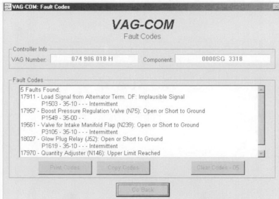
Fig 7 Fault codes screen
