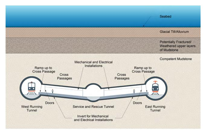
Figure 9: Indicative tunnel cross-section.
