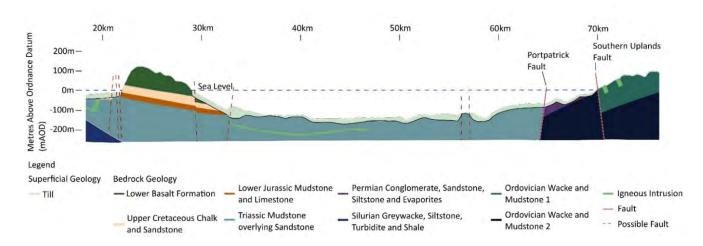
Figure 7: Longitudinal section through indicative tunnel alignment.
