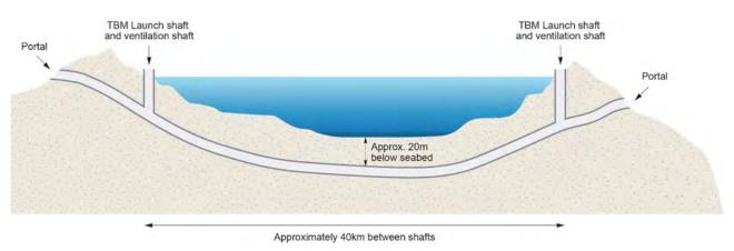
Figure 8: Indicative tunnel vertical alignment.
