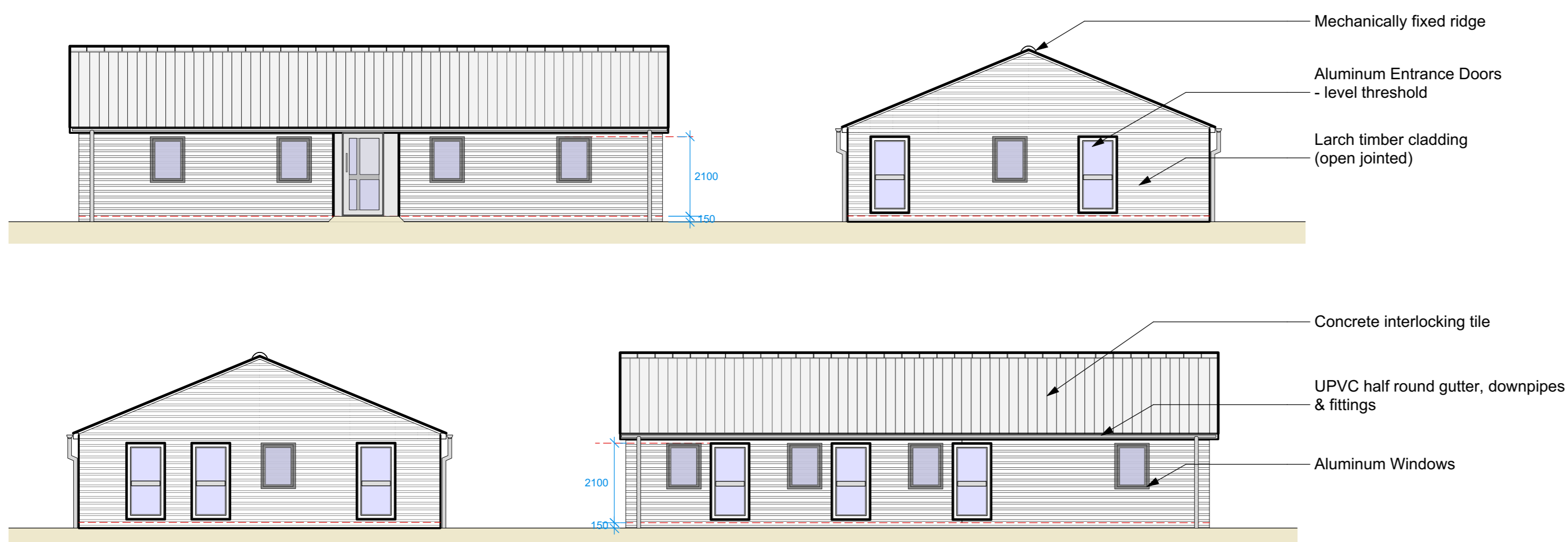
PROPOSED ELEVATIONS (SCALE 1:100)
