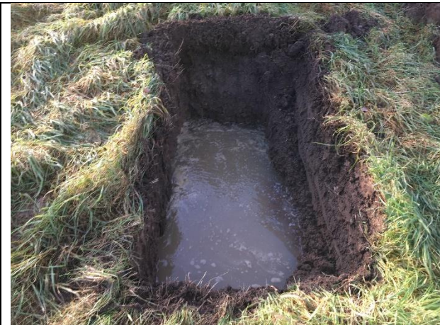
Plate 21 – Perched water flowed into shallow excavations from the glacial soils, as evidenced at VP2 (left) and DR2 (right) in the southern paddock.
