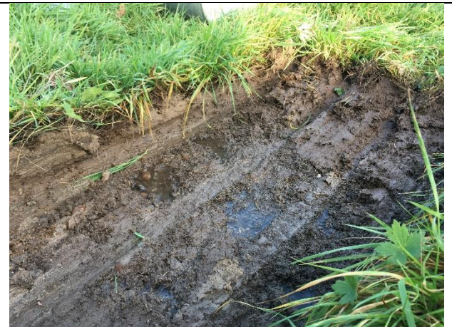
Plate 21 – Perched water flowed into shallow excavations from the glacial soils, as evidenced at VP2 (left) and DR2 (right) in the southern paddock.
