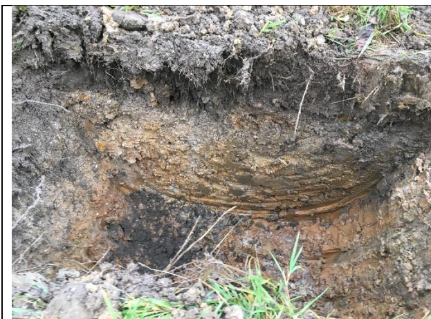
Plate 29 – Slightly sandy slightly gravelly Clay, exposed in SA4 in the E of the site.
