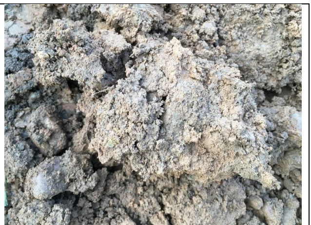
Plate 30 – Soft grey-brown slightly sandy slightly gravelly Clay, recovered from SA4 at c.0.5m.
