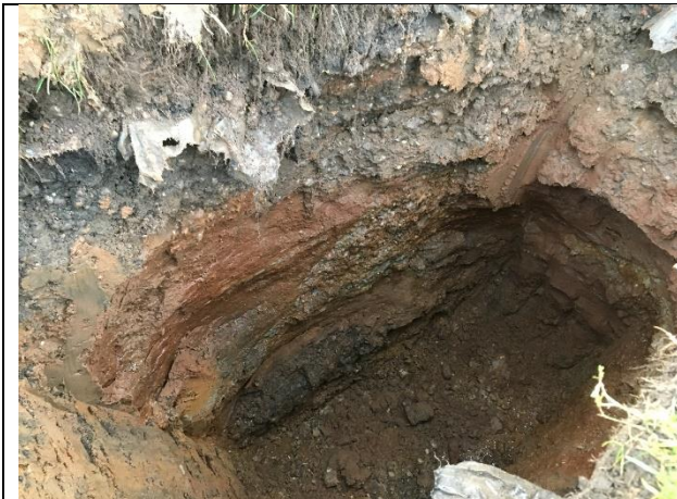
Plate 27 – The glacial soils were variable in composition, noted in TP1 with very clayey Sand interspersed with very sandy Gravel.
