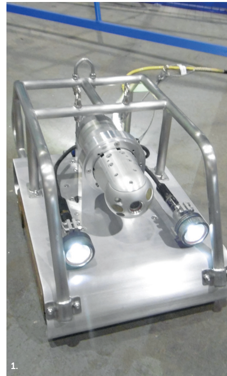
1. ROV for visual inspection of store.
