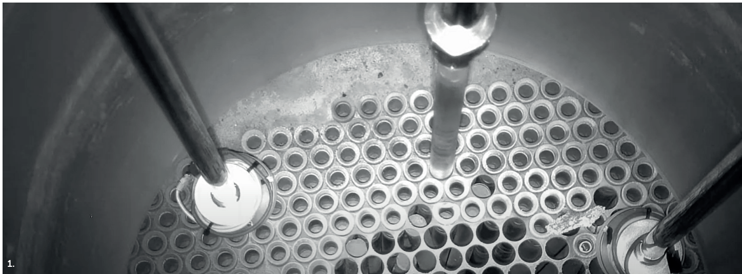
1. Camera footage within Dounreay Fast Reactor showing breeder elements and damage to top plate (© DSRL)
