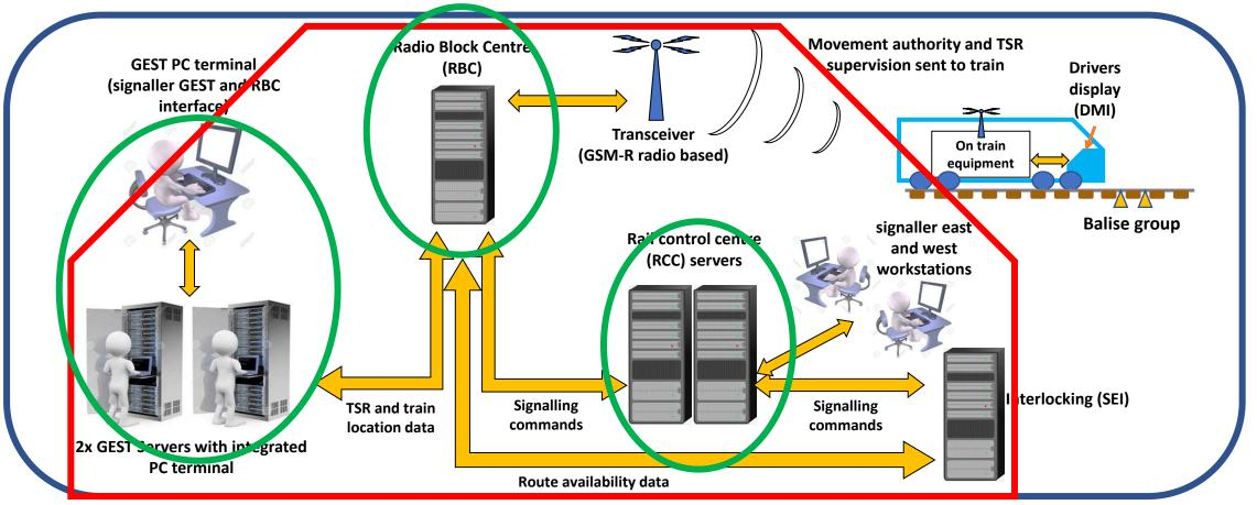
**ERTMS system** = hardware, software, data relating to train control **Sub-systems = part of the bigger system, but which is itself a system**
