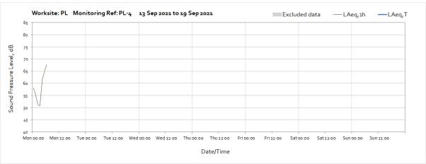
Note: Missing data between 07:00 on Monday 13<sup>th</sup> September and 00:00 on 1<sup>st</sup> November was due to insufficient solar power to recharge the battery after the relocation of the monitor on the 20<sup>th</sup> of August. The monitor will be relocated back to the original location to avoid loss of information in the future.
