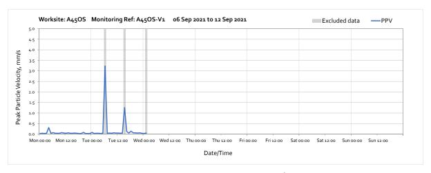
Note: The vibration monitor was decomissioned from site at 02:00 on 8<sup>th</sup> September 2021. The high vibration levels measured were due to local interference of the monitoring station
