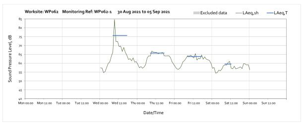
Note: Missing data between 01:00 on Sunday 5<sup>th</sup> September and 14:00 on Monday 6<sup>th</sup> September was due to loss of power at the monitoring station due to vegetation growing around the equipment and obscuring the solar panel. The vegetation has since been cut down to avoid power outages in the future.
