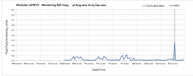
Note: High vibration levels measured at 14:00 on Sunday 5<sup>th</sup> September 2021 were due to due to local disturbance at the monitor station and not representative of HS2 vibration levels at the nearest receptor.
