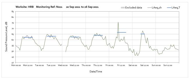
Note: Missing data from 00:00 until 03:00 on Wednesday 22<sup>nd</sup> September was due to a memoty fault within the monitoring station. The monitor firmware will be updated with view of avoiding further loss of data.
