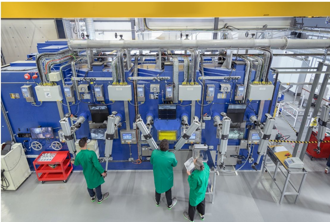
Figure 10 – UKAEA’s Materials Research Facility (MRF) prepares and examines samples of radioactive materials to assess their performance 24
