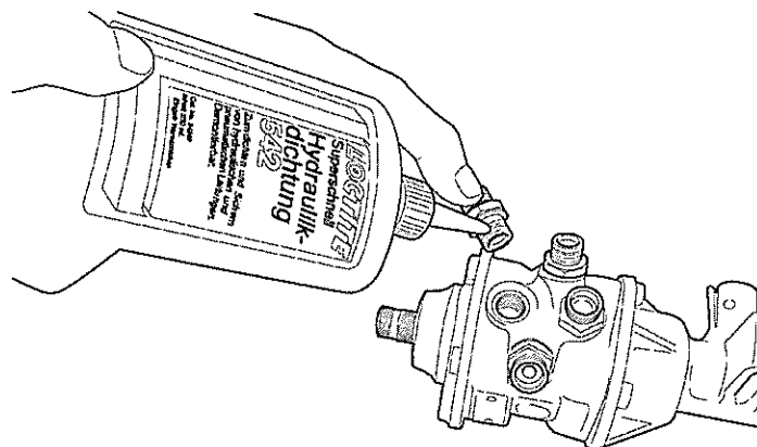
Fig 14 Refitting stud couplings using Loctite 542
