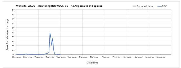
Note: High levels of vibration measured through out the week were due to earthworks and bentonite slab constuction carried out in the vicinity of the monitor. The nearest residential receptors are further from the works and vibration levels at the receptor will therefore be lower.
