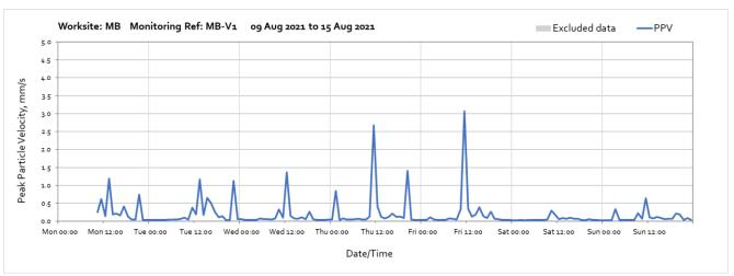
Note: Missing data between 16:00 on Friday  $6^{th}$  August and 10:00 on Monday  $9^{th}$  August 2021 was due to a software issue at the monitoring station. High vibration levels measured across the week were due to earthworks undertaken near to the monitoring location. The nearest residential receptors are further away from the works and vibration levels at the receptors will therefore be lower.
