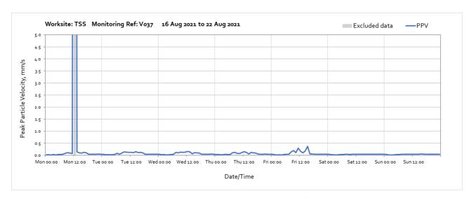
Note: High vibration levels measured from 12:00 until 13:00 on Monday  $16^{th}$  August were due to local interference during routine maintenance of the monitor.
