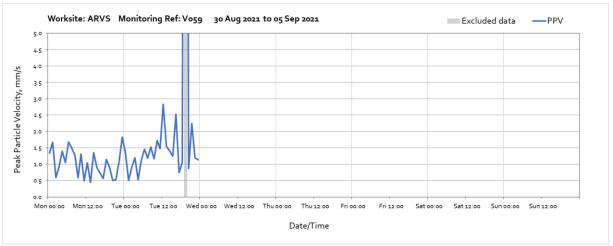
Note: High vibration levels measured from 19:00 until 20:00 on Wednesday 30<sup>th</sup> August were due to local interference of the monitor and are not representative of HS2 vibration levels at the receptor.
