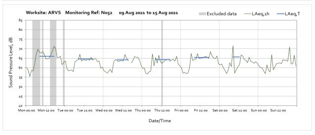
Note: Missing data from 16:00 until 17:00 on Wednesday 11<sup>th</sup> August was due to a memory card error. The memory card has been reformatted with view of avoiding further loss of data.
