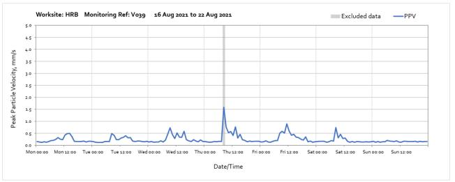
Note: High vibraton levels measured from 08:00 until 09:00 on Thursday 19<sup>th</sup> August were due to local interference of the monitor and are not representative of HS2 vibration levels at the receptor.
