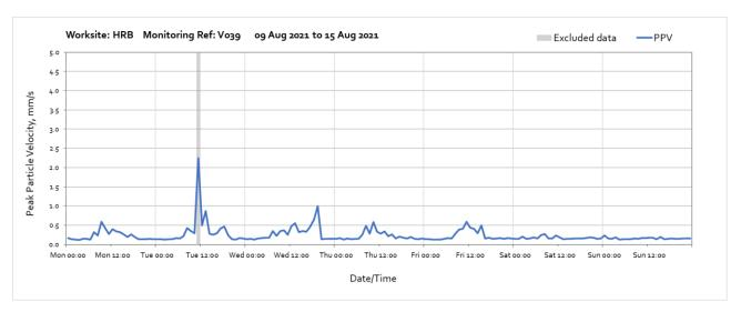
Note: High vibraton levels measured from 11:00 until 12:00 on Tuesday 10<sup>th</sup> August were due to local interference of the monitor and are not representative of HS2 vibration levels at the receptor.
