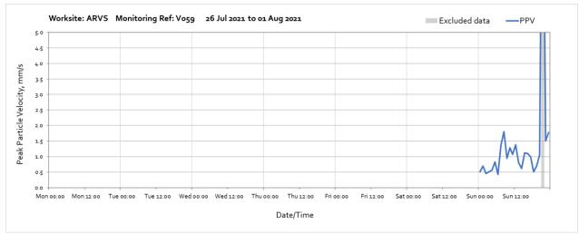
Note: High vibration levels measured from 21:00 until 22:00 on Sunday 1<sup>st</sup> August were due to local interference of the monitor and are not representative of HS2 vibration levels at the receptor.
