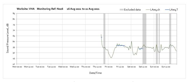
Note: Missing data from 12:00 on Friday 13<sup>th</sup> August until 15:00 on Thursday 19<sup>th</sup> August was due to a memory card error. The memory card was reformatted however the memory subsequently failed. The monitor was replaced with view of minimising further loss of data.
