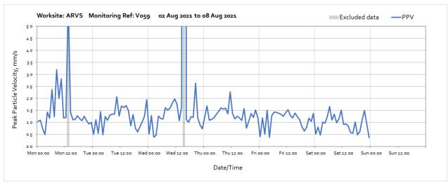
Note: High vibration levels measured from 13:00 until 14:00 on Monday 2<sup>nd</sup> August and from 15:00 until 16:00 on Wednesday 4<sup>th</sup> August were due to local interference of the monitor and are not representative of HS2 vibration levels at the receptor. Missing data from 00:00 on Sunday 8<sup>th</sup> August until 16:00 on Tuesday 10<sup>th</sup> August was due to depletion of the monitoring station battery caused by a delay in conformation of access to replace the battery.
