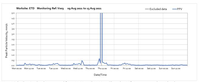
Note: High vibration levels measured from 11:00 until 12:00 on Thursday 12<sup>th</sup> August were due to local interference during routine maintenance of the monitor.
