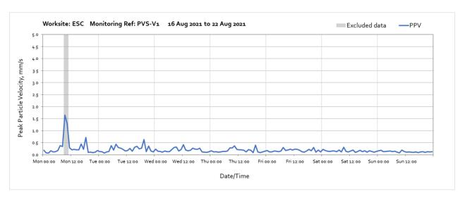
Note: High vibraton levels measured from 09:00 until 11:00 on Monday 16<sup>th</sup> August were due to local interference of the monitor and are not representative of HS2 vibration levels at the receptor.
