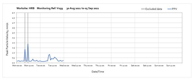
Note: High vibraton levels measured from 08:00 until 09:00 and 11:00 until 12:00 on Monday 30<sup>th</sup> August were due to local interference of the monitor and are not representative of HS2 vibration levels at the receptor.
