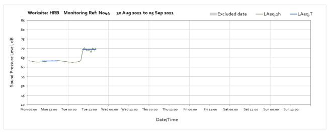
Note: Continuous noise levels measured throughout the week were caused an operational generator near to the monitor.
