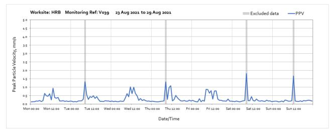
Note: High vibraton levels measured throughout the week were due to local interference of the monitor and are not representative of HS2 vibration levels at the receptor.
