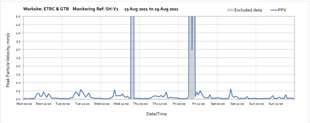
Note: High vibration levels measured from 19:00 until 20:00 on Wednesday 25<sup>th</sup> August and from 07:00 until 10:00 on Friday 27<sup>th</sup> August were due to local interference of the monitor and are not representative of HS2 vibration levels at the receptor.
