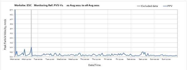
Note: High vibraton levels measured from 00:00 until 01:00 and 17:00 until 18:00 on Monday  $2^{nd}$  August were due to local interference of the monitor and are not representative of HS2 vibration levels at the receptor.
