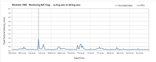
Note: High vibraton levels measured from 08:00 until 09:00 on Tuesday 3<sup>rd</sup> August were due to local interference of the monitor and are not representative of HS2 vibration levels at the receptor.
