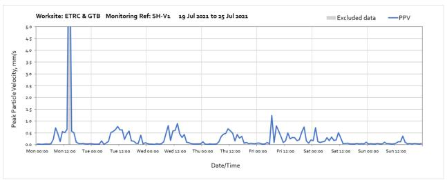
Note: High vibration levels measured from 14:00 until 15:00 on Monday 19<sup>th</sup> July were due to local interference of the monitor and are not representative of HS2 vibration levels at the receptor.
