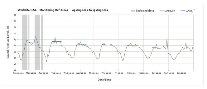
Note: Missing data from 12:00 until 16:00 on Thursday 12<sup>th</sup> August was due to a fault with the monitoring station server connection. The memory card was reformatted with view of avoiding further loss of data.
