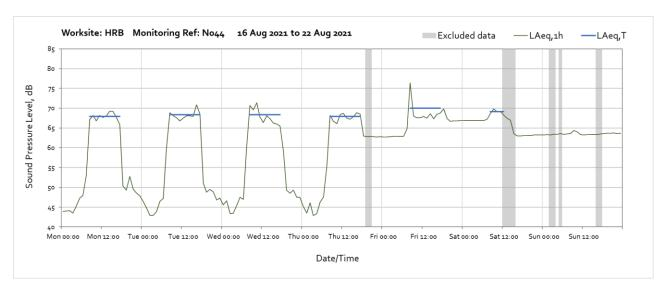
Note: Continuous noise levels measured throughout the week were caused an operational generator near to the monitor.
