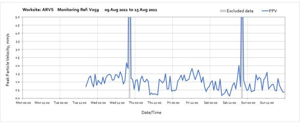
Note: High vibration levels measured from 20:00 until 21:00 on Wednesday 11<sup>th</sup> August and from 20:00 until 21:00 on Saturday 14<sup>th</sup> August were due to local interference of the monitor and are not representative of HS2 vibration levels at the receptor. Missing data from 00:00 on Sunday 8<sup>th</sup> August until 16:00 on Tuesday 10<sup>th</sup> August was due to depletion of the monitoring station battery caused by a delay in confirmation of access to replace the battery.
