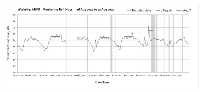
Note: Missing data from 00:00 until 10:00 on Wednesday 18<sup>th</sup> August was due to a memory card error. The memory card has been reformatted with view of avoiding further loss of data.
