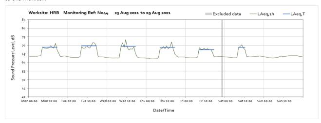
Note: Continuous noise levels measured throughout the week were caused an operational generator near to the monitor.
