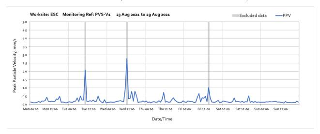
Note: High vibration levels measured throughout the week were due to local interference of the monitor and are not representative of HS2 vibration levels at the receptor.
