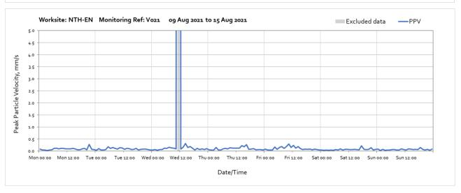
Note: High vibration levels measured from 11:00 until 12:00 on Wednesday 11<sup>th</sup> August were due to local interference during routine maintenance of the monitor.
