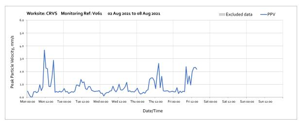
Note: Missing data from 16:00 on Friday 6<sup>th</sup> August until 18:00 on Tuesday 10<sup>th</sup> August was due to depleted batteries and difficulty in obtaining access to change the batteries due to the school holidays. A temporary additional vibration monitor V061 (temp) was installed within CRVS worksite 4 metres from vibration monitor V061 on Tuesday 10<sup>th</sup> August to provide cover for vibration monitor V061.
