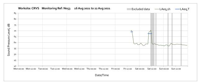
Note: Missing data from 00:00 on Sunday 15<sup>th</sup> August until 15:00 on Friday 20<sup>th</sup> August was due to equipment failure during software upgrade and error with the SD card. The unit was replaced to prevent further loss of data.
