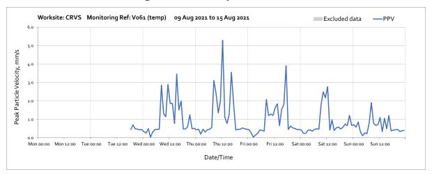
Note: A temporary additional vibration monitor V061 (temp) was installed within CRVS worksite 4 metres from vibration monitor V061 on Tuesday  $10^{th}$  August. It was installed to provide cover for vibration monitor V061 because it ran out of battery on the  $6^{th}$  of August and there was difficulty in obtaining access to change the batteries due to the school holidays.
