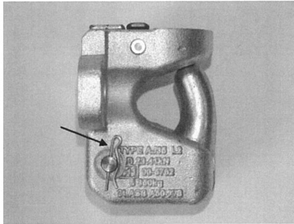
Fig 1 Removal of the 'R' Clip
