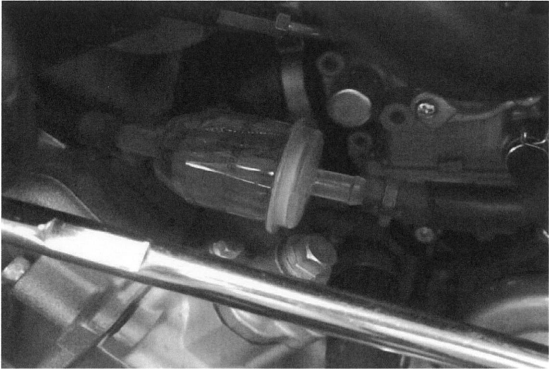
Fig 6 Fuel Filter Fitted and In Position
