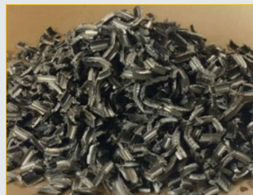
ILW Magnox fuel cladding swarf
