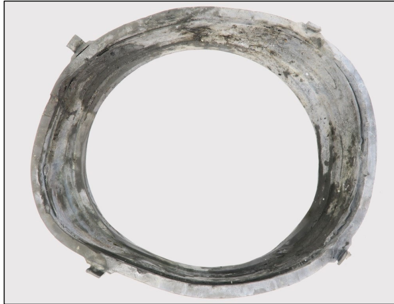
Figure 23 Energy absorbing ring (Front view) (Image used with permission of Rolls-Royce PLC)
