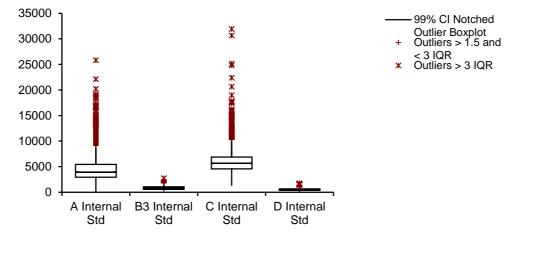
The table and graph show the results obtained for the internal standard at each of the sites. All results are calculated as area under peak with the exception of site B. Site B utilized the Cliquid Chemoview<sup>TM</sup> software (AB Sciex) which derives an average ion count. Site B data is therefore not comparable to the other three sites. Site D (Waters Premier) shows a significantly reduced signal (mean = 526) compared to the other two sites (AB Sciex 4000, Waters Xevo TQS).
