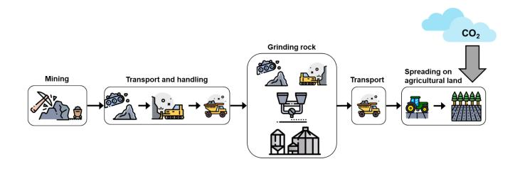
Figure 12: Illustrative flow diagram of an archetypal enhanced weathering (EW) value chain. Here, carbonate-able minerals, such as basalt or olivine, are mined, and then processed to produce a fine powder, which can be then transported and spread on available land. Subsequently, the carbonation of this material proceeds as a function of particle size, temperature, water, and time. CO2 removed in this manner can be considered to be permanently removed.
