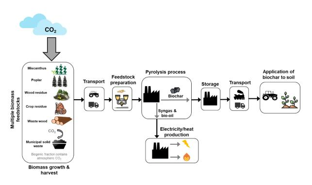
Figure 14: Illustrative flow diagram of an archetypal biochar value chain. The initial cultivation and growth of the biomass absorbs CO2 from the atmosphere. The biomass is then processed and fed to a pyrolysis process, which produces both biochar and a range of co-products, which can be used for the provision of energy services. The biochar is then subsequently incorporated with the soil where it decays over time as a function of the pyrolysis process conditions and prevailing soil conditions.
