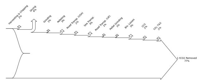
Figure 10: Illustrative carbon removal efficiency diagram for a UK BECCS project using biomass imported from the USA. This example assumes 98% CO2 capture. At 90% capture rate, the carbon removal efficiency is reduced to approximately 70%.
