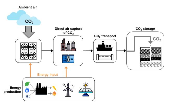
Figure 9: Illustrative flow diagram of an archetypal direct air carbon capture and storage (DACCS) value chain. Here the CO2 is directly removed from ambient air, and subsequently transported to a geological storage facility.
