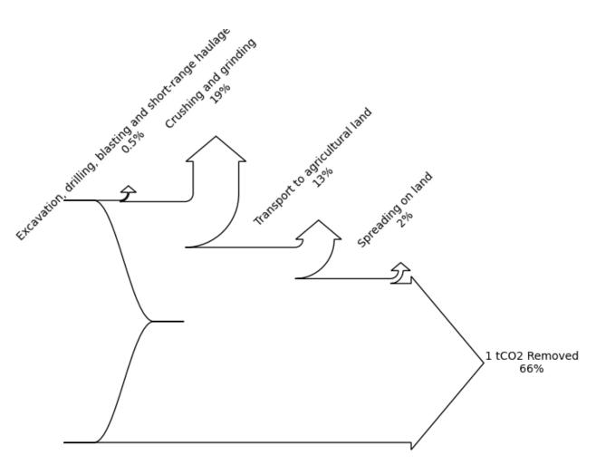
Figure 13: Illustrative carbon efficiency of passive enhanced weathering process. Here it is assumed that the mineral material is available in the UK. It can be observed that the primary sources of carbon leakage are the energy required for mineral size reduction, transport, and spreading on land.
