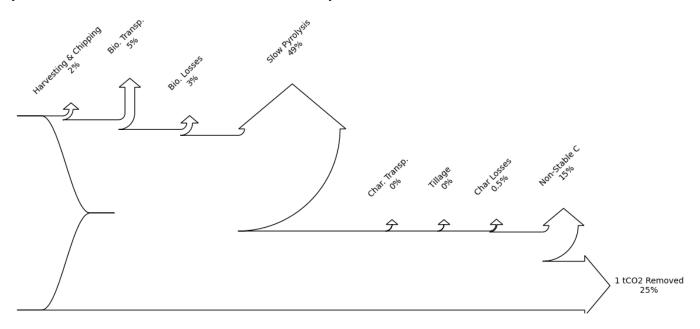
Figure 15: Illustrative carbon removal efficiency diagram for biochar application in the UK using forest residue from Scotland with char application in the midlands.
