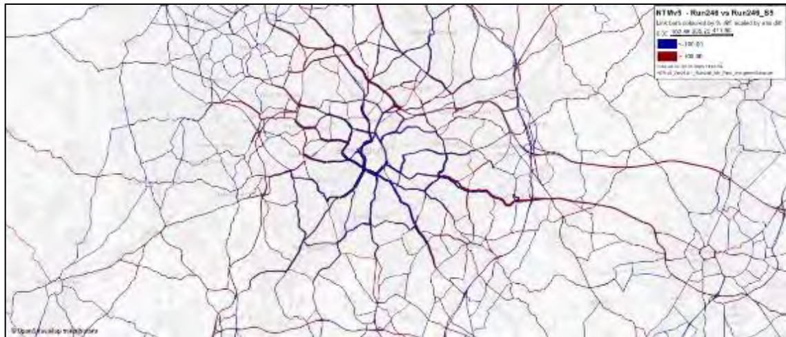
Figure 7.11: Flow differences in Birmingham between the baseline run and the sensitivity test 5 model run
