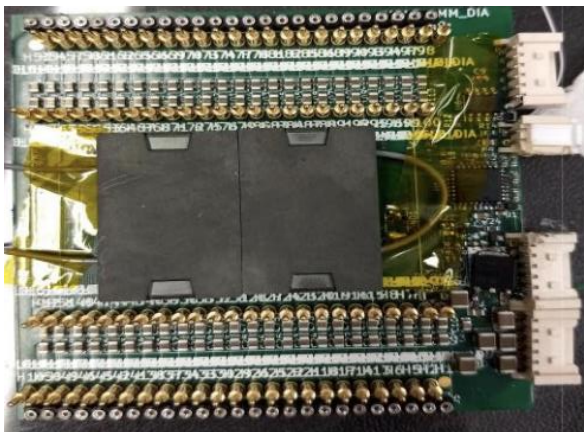
The proposed power converter module with an integrated gate drive circuitry
