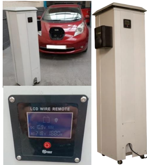
Portable and modular 12.5kWh battery storage prototype charging system with both AC & DC charging capability (see display).
