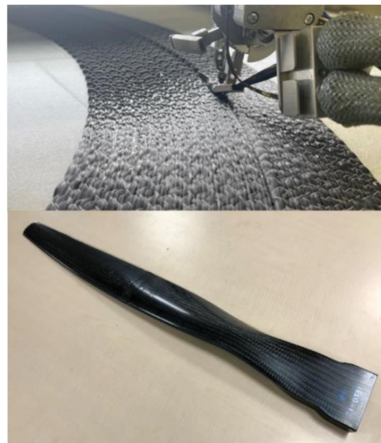
Fibre placement process (top) and prototype UAM blade (bottom).
