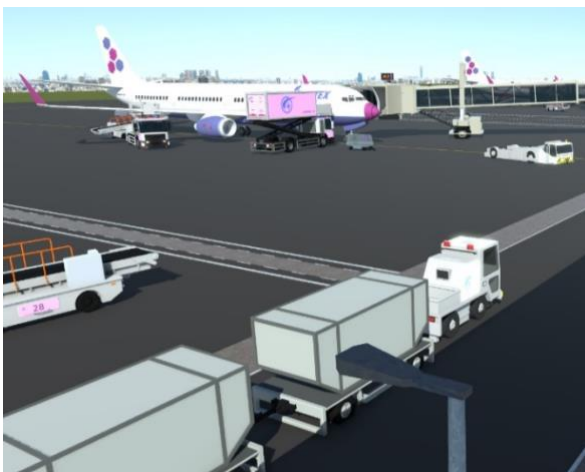
Screenshot from the simulator showing an autonomous baggage tug navigating the airport as part of the virtual test drive
