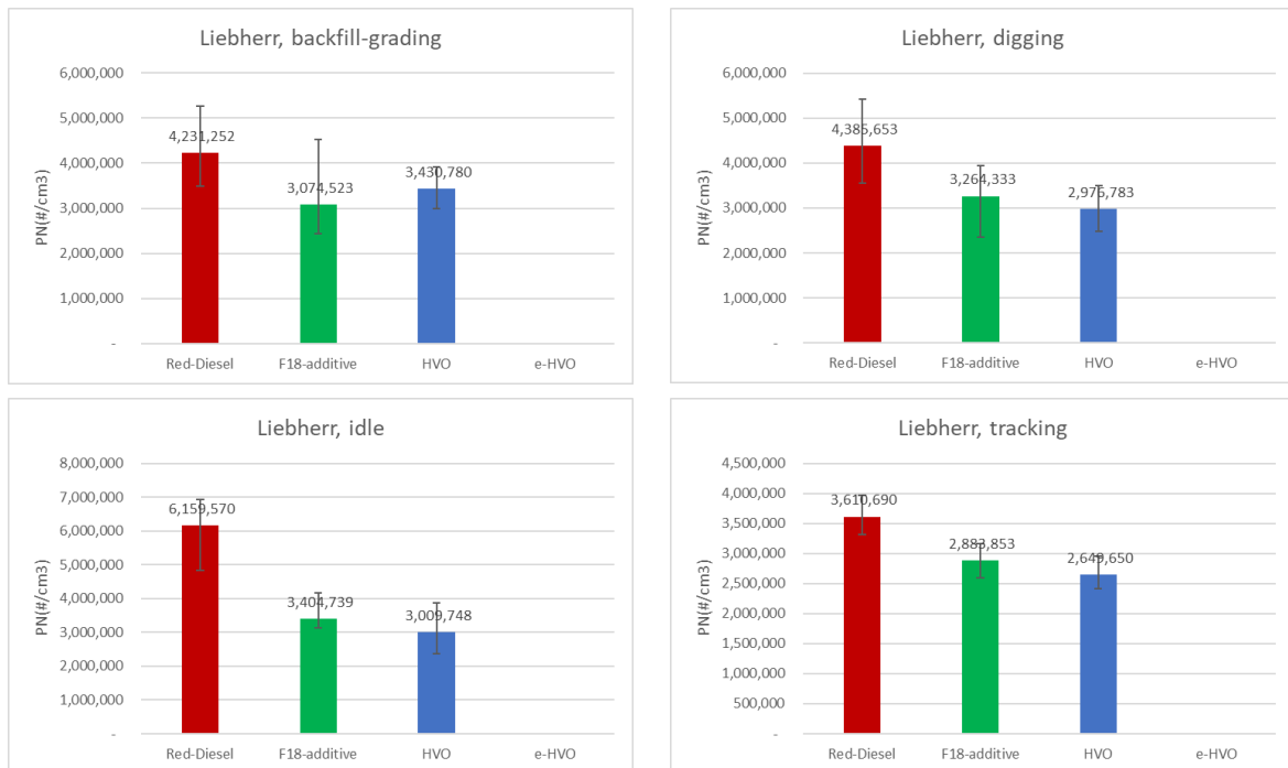
Figure 6 Bar charts of PN emissions (Liebherr) comparing Red-Diesel with F18-additive, HVO, and enhanced HVO (e-HVO). Red-Diesel is plotted in red, F18 additive in green, HVO in blue and enhanced HVO (e-HVO) in yellow.
