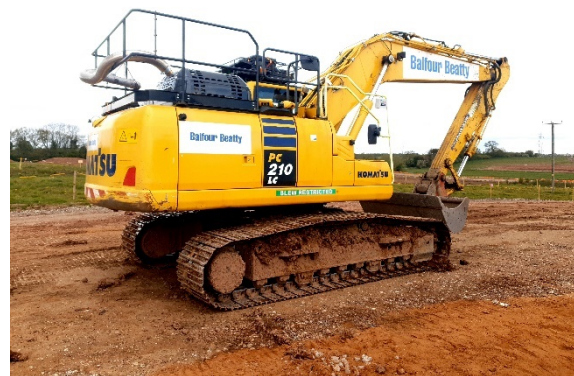
Figure 2 Komatsu PC210 tracked excavator.
