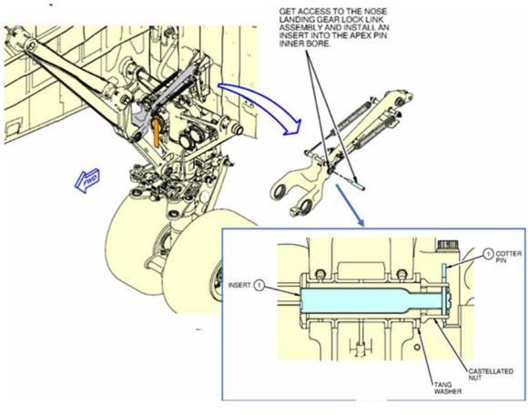
Figure 4 Installation diagram of NLG apex pin inner bore insert
