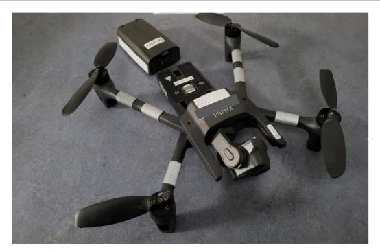
**Figure 1** UA showing damage to rotor and dislodged battery
