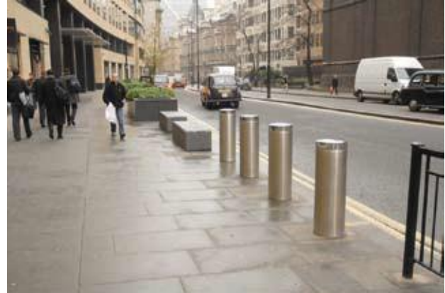
Figure 2.4 Use of planters, structures, bollards and pedestrian guardrailing for security purposes and also to deter pavement parking
