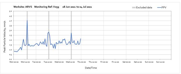
Note: High vibration levels measured throughout the week were due to local intereference of the monitor and are not representative of HS2 vibration levels.
