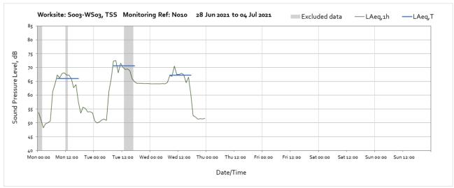
Note: Continuous noise levels measured outside of core construction hours were due to refridgeration plant equipment associated with a nearby hotel and is not associated with HS2 contruction.
