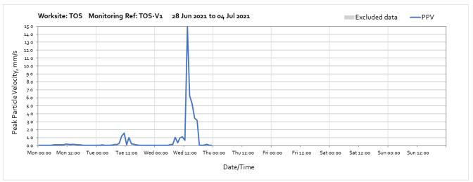
High vibration levels between 08:00 and 18:00 on Wednesday 30<sup>th</sup> June were due to work activities (ground raking works and removal of existing concrete slab) undertaken near the monitor location. The nearest residential receptors are further away from the works and vibration levels at the receptors will therefore be lower.
