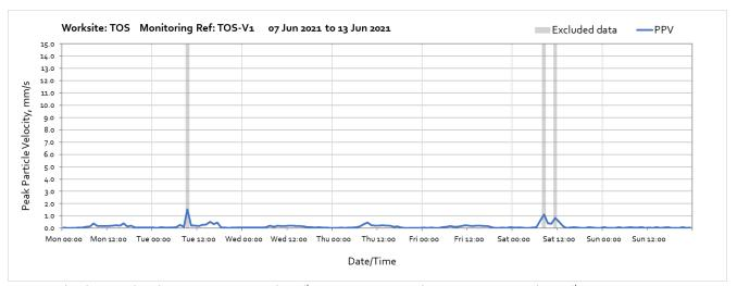
Note: High vibration levels at 09:00 on Tuesday 8<sup>th</sup> June; at 08:00 and at 11:00 on Saturday 12<sup>th</sup> June; were due to local interference of the monitor and not reppresentative of HS2 vibration levels.
