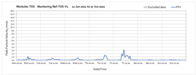
High vibration levels measured between 08:00 and 17:00 on Friday 25<sup>th</sup> June were due to excavaction works undertaken near the monitoring location. The nearest residential receptors are further away from the works and vibration levels at the receptors will therefore be lower.
