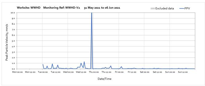
Note: High vibration levels at 09:00 on Tuesday 1<sup>st</sup> June; at 12:00, at 15:00 and 22:00 on Wednesday 2<sup>nd</sup> June were due to local interference of the monitor and are not representative of HS2 vibration levels at nearby receptors.
