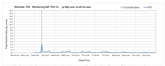
Note: High vibration levels at 08:00 on Tuesday 1<sup>st</sup> June were due to local interference of the monitor and not reppresentative of HS2 vibration levels.
