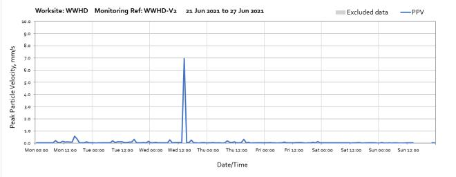
Note: High vibration levels at 14:00 on Wednesday 23<sup>rd</sup> June were due to earthworks undertaken near to the monitor location. The nearest residential receptors are further away from the works and vibration levels at the receptors will therefore be lower. Missing data between 15:00 and 22:00 on Sunday 27<sup>th</sup> June were due to lost of signal.
