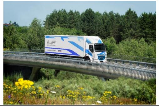
Figure 1 DAF LF Electric, a nineteen tonne battery electric HGV
