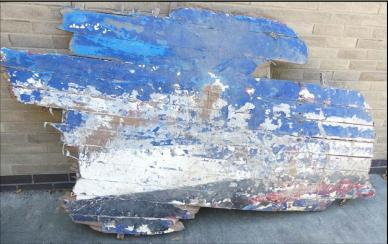
Figure 3: Recovered wreckage section
