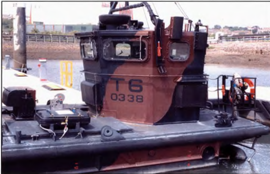
Figure 1.4.18 – LCVP Mk5B Wheelhouse viewed from the Port Side.
