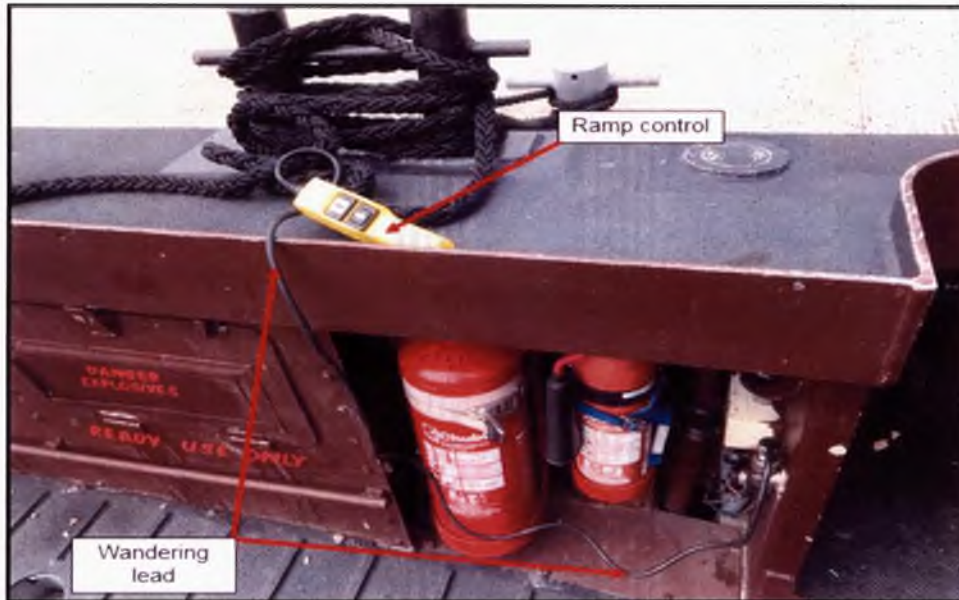
Figure 1.4.16 – LCVP Mk5B Ramp Operating Control on the Starboard Side viewed from the Rounddown.
