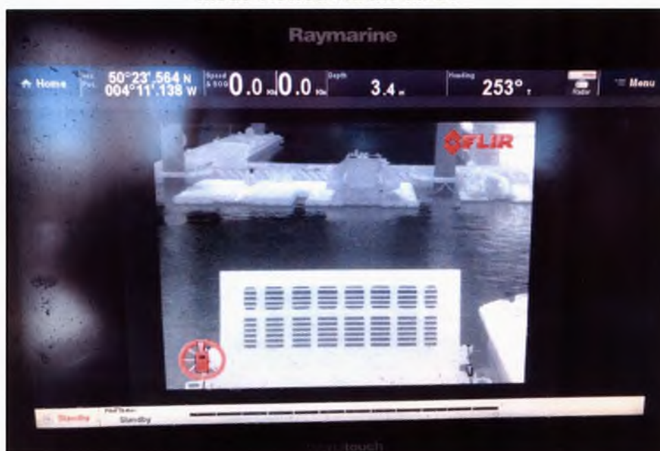
Figure 1.4.26 – LCVP Mk5B Camera view in Visible Daylight Mode viewed via the MFD.
