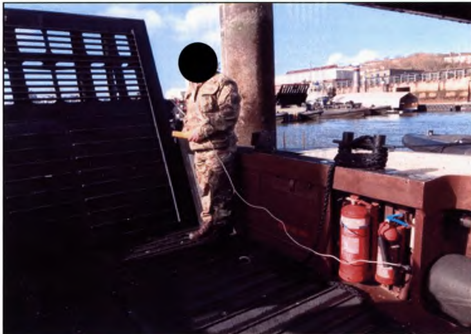
Figure 1.4.17 – Operating the Ramp using the Wandering Lead at maximum length.
