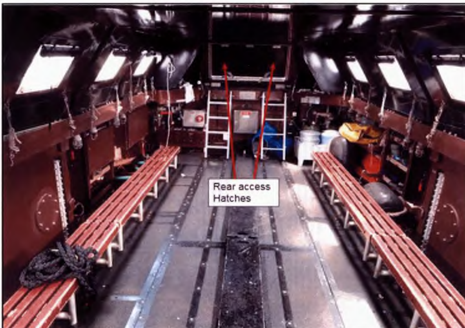
Figure 1.4.13 – LCVP Mk5B Welldeck viewed from Forward looking Aft with the Centre Benches Collapsed.
