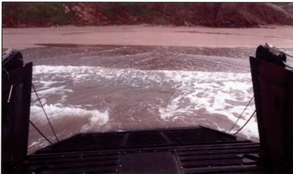
Figure 1.4.15 – LCVP Mk5B with Ramp lowered onto a Beach.
