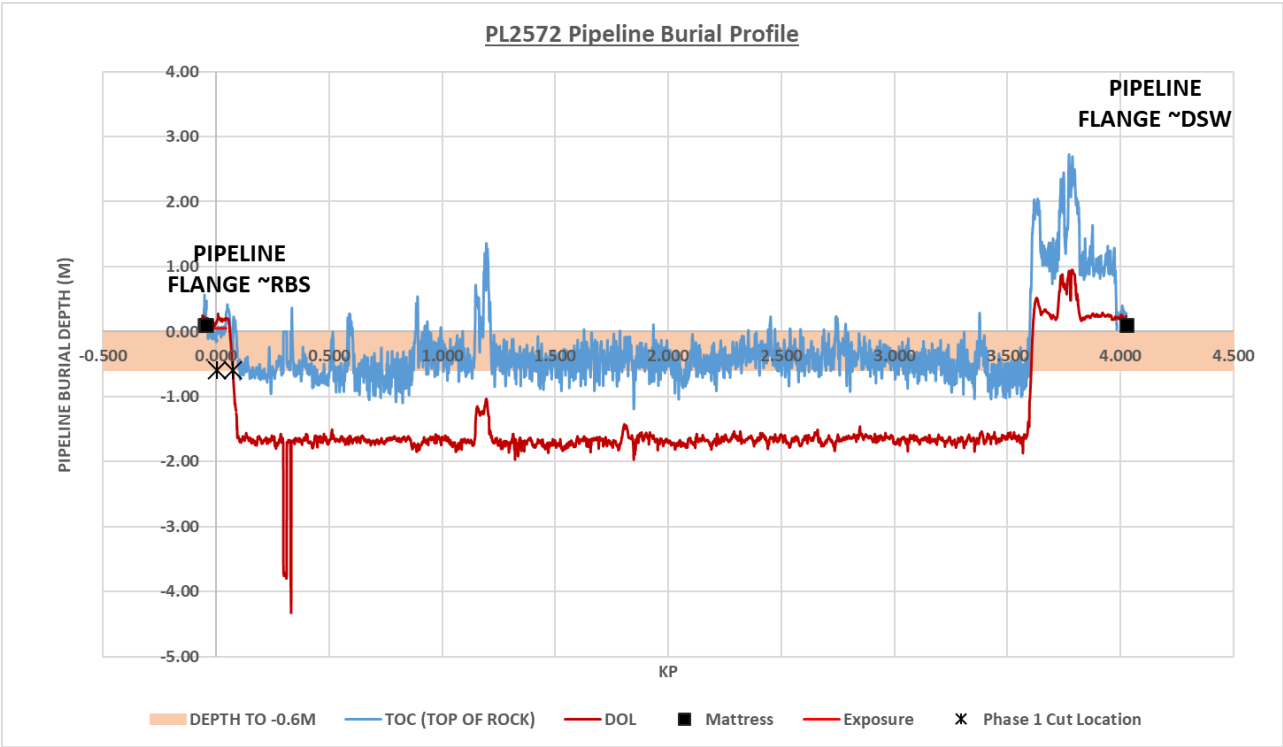
Figure E.2.2: PL2572 depth of burial profile
