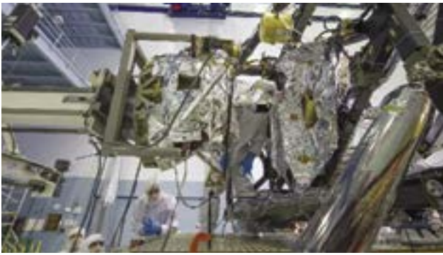
Installation of MIRI into the instrument module
