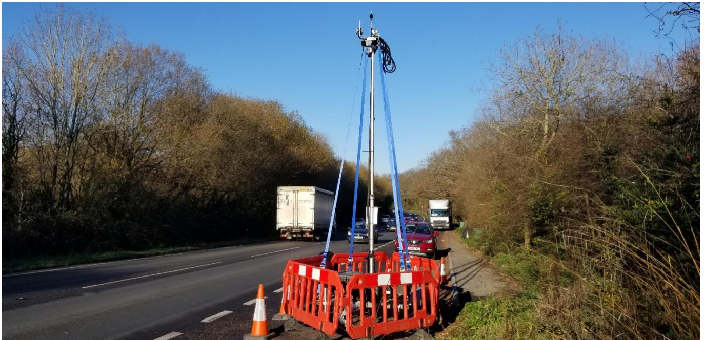
Figure 4.4. Noise camera installed on the A326 Marchwood Bypass
