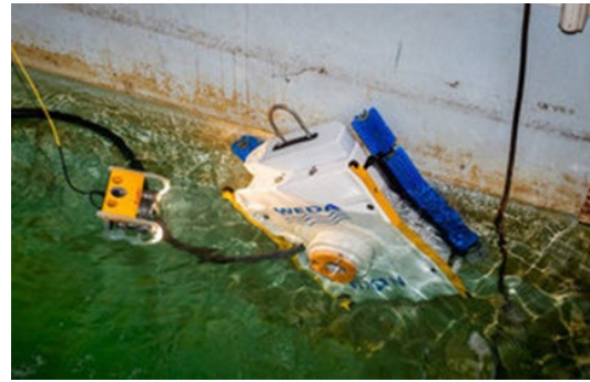
Figure 32: Trials of an adapted swimming pool cleaner to clean surfaces in PFSP
