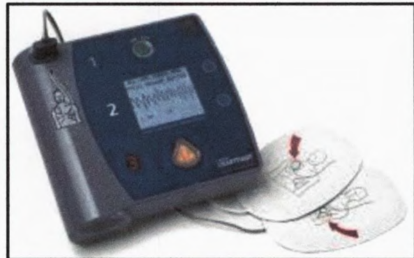
Figure 13: HeartStart FR2+ front panel
