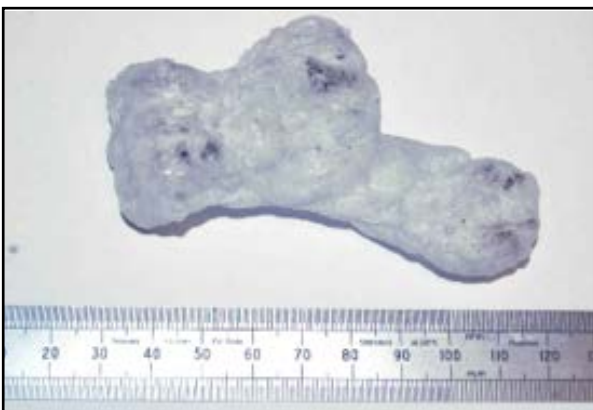
Figure 8: Styrene residue sample
