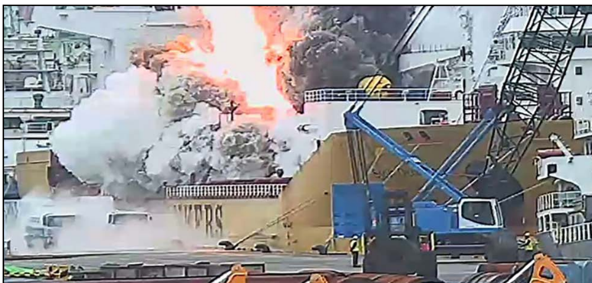
Figure 5: CCTV still showing vapour ignition
