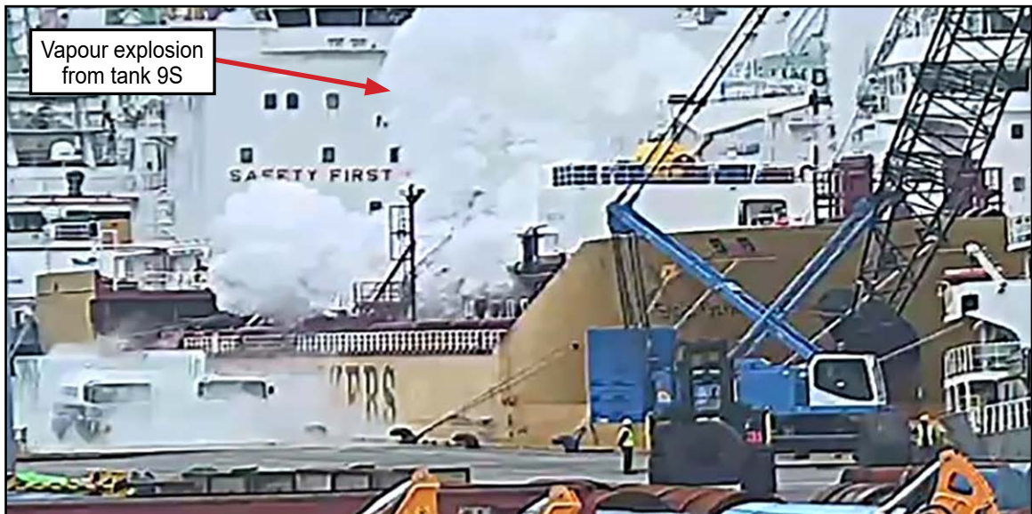
Figure 4: CCTV still showing tank rupture and vapour release
