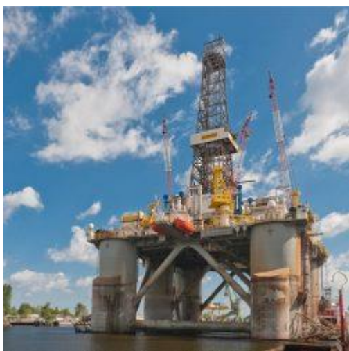
Figure 3.8 – Typical semi-submersible rig 9
