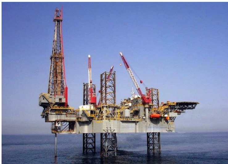
Figure 3.6 – Typical jack-up rig
